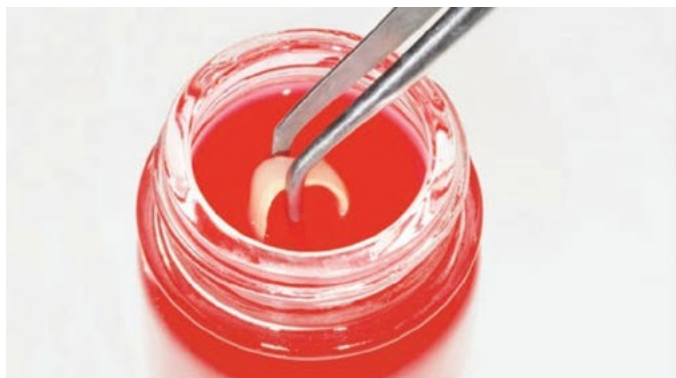
Fig. 14 and 15 Inspection of the complete sealing of the sintered joint using a colour penetration test.
