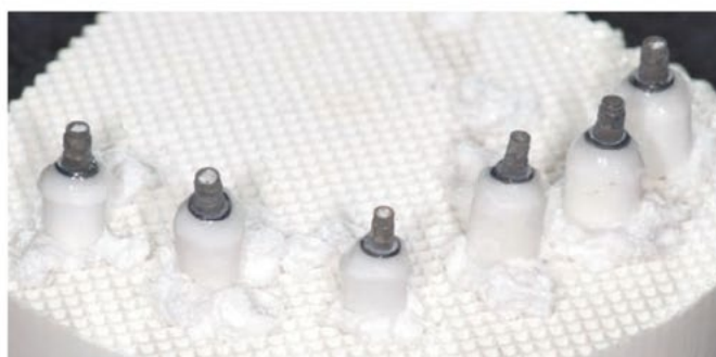
Fig. 14 Successful production of hybrid abutments.
