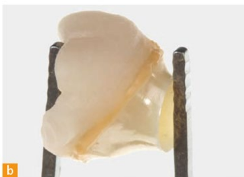
Fig. 9a and b Clamping bracket of the two sintered composite components during the furnace sintering.
